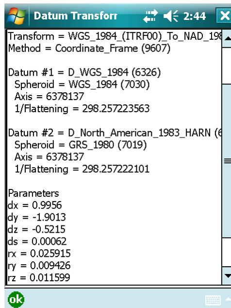
Since this is not an ITRF 00 to NAD 83 (CORS96) transformation, it could introduce 5-7cm of error.
