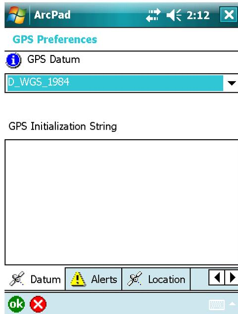
The output datum is specified in the .prj file used by ArcPad to set the Map Projection. The .prj file used will be that .prj associated with the first layer loaded in the current map, the ArcPad.prj file found in \My Documents (if present), or the .prj file chosen in the Table of Contents. Press the 'Map Properties' button to view current map projection information (last page), including the datum being used in the map.
